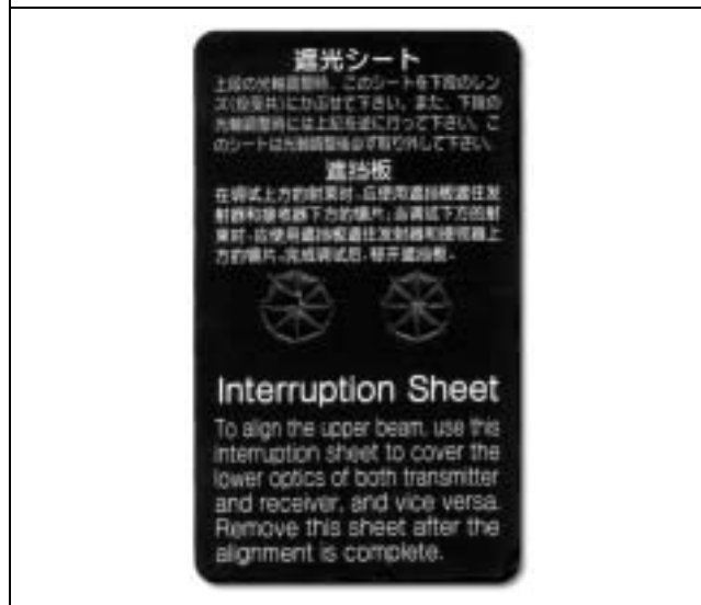
Figure 19: Alignment Interruption Sheet
