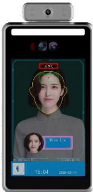
The 8" IPS touchscreen gives clear verbal and on-screen directions when guests are registering their arrival, and will register the temperature of the person in it's integral database, or it can be integrated in to a 3<sup>rd</sup> party database via RS485, Wiegand, or USB.
