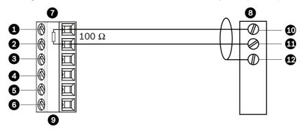
Figure 3.2 Connections for Biphase Operation
