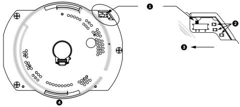
Figure 3.9 Position of CPU Switch for RS232 Operation
