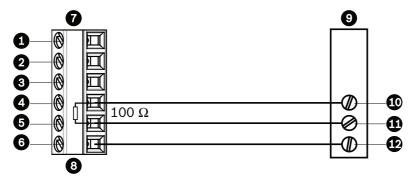
Figure 3.6 Connections for RS485 Operations
