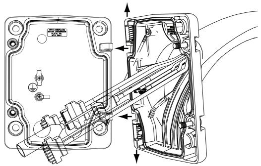
Figure 2.2 Connect Pendant Arm to Mounting Plate
