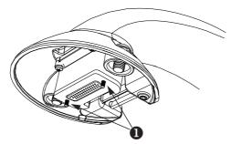
If your pendant arm contains these pins, **DO NOT** attempt to mount a Pressurized Environmental Housing to the mount. You must order the appropriate mounting option for the Pressurized Environmental Housing.
