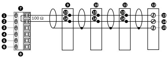
Figure 3.3 Connections for a Daisy Chain Configuration
