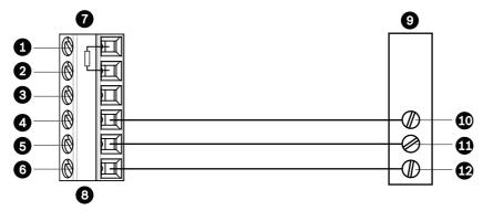
Figure 3.4 Connections for RS232 Operation
