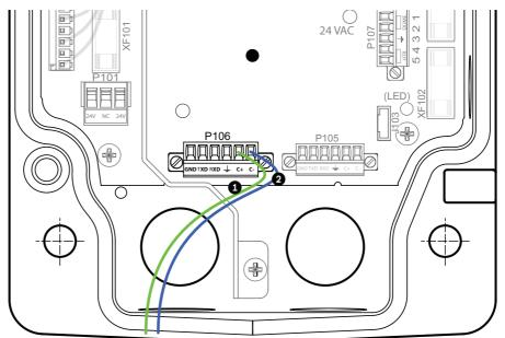
Figure 3.8 Detail of P106 Connections
