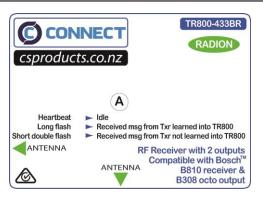
The TR800-433BR is a 433MHz radio receiver compatible with the Bosch™ Solution 2000/3000 series of intruder alarm panels. It emulates a Bosch RADION B810 Receiver and also provides four outputs by emulating a Bosch B308 Octo Output Module.
