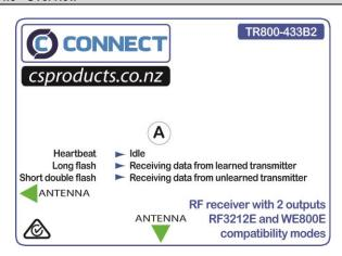
The **TR800-433B** (is a 433MHz radio receiver compatible with the Bosch series of intruder alarm panels. Note **TR800-433B2** is the same as **TR800-433B**.
