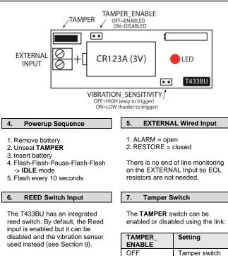
To restore the REED input, bring the magnet in proximity to the T433BU. To activate the REED input, remove the magnet.
